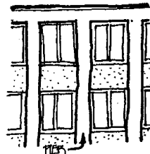
Piers and Spandrels
